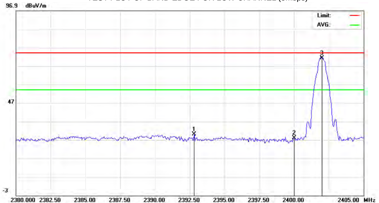
TEST PLOT OF BAND EDGE FOR LOW CHANNEL (3Mbps)
