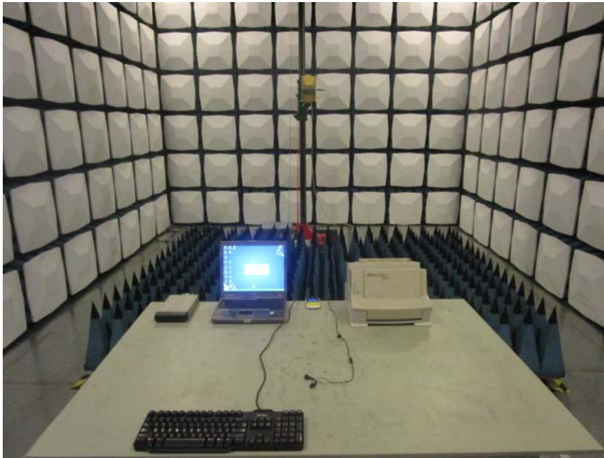
Radiated Emission –Front View (Above 1 GHz)
