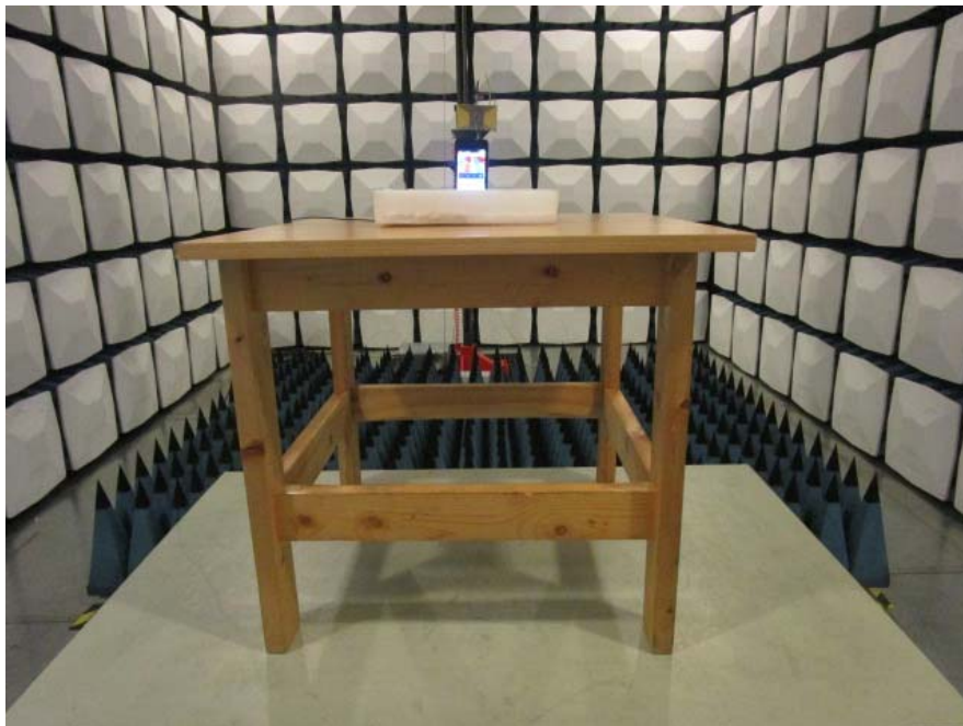
Radiated Emission View---Above 1GHz
