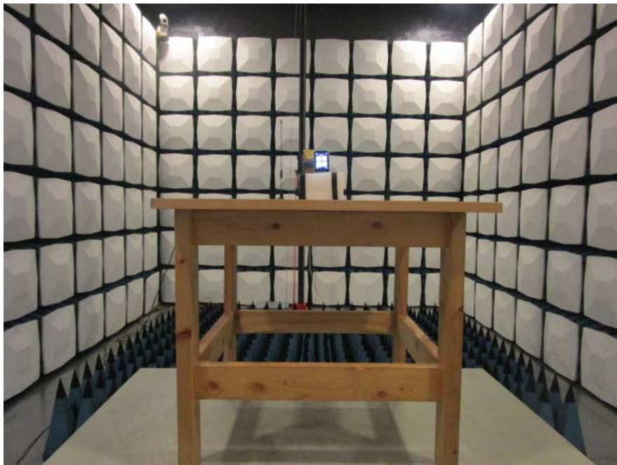
Radiated Emission View---Above 1GHz
