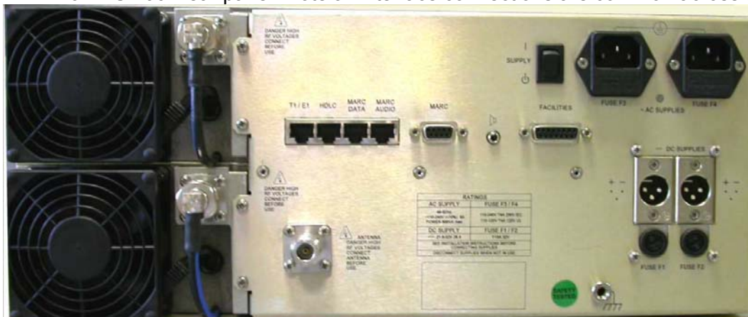
T6T HS 100 Rear panel. Note all interface connections are common across the range.
