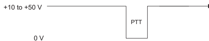
+10 to +50 Volt Keying with Negative Going Active Signal
