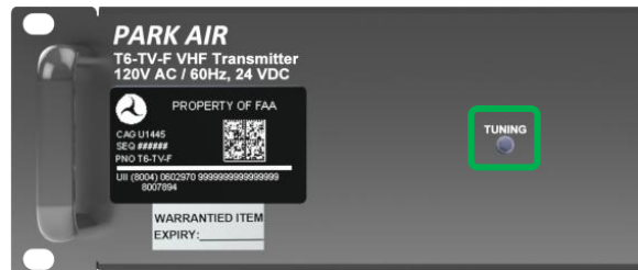
Figure 6-5. Tuning Port Location
