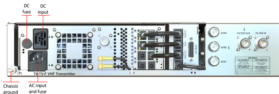
Figure 7-5. Fuse Locations on Rear of T6F Transmitter
