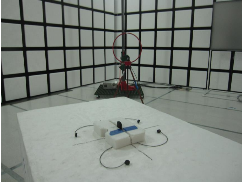
RADIATED BACK PHOTO (BELOW 30MHz)
