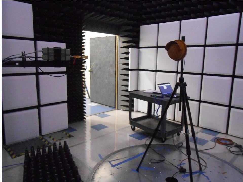
Radiated Emissions Test set up 50 – 75 GHz (2)
