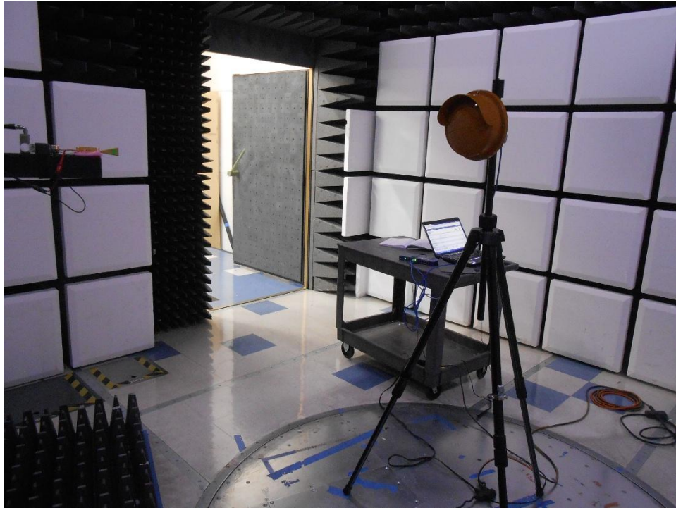
Radiated Emissions Test set up 30 - 1000 MHz (2)
