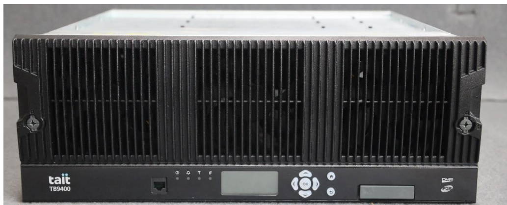
Photograph 01: Base station – Front view
