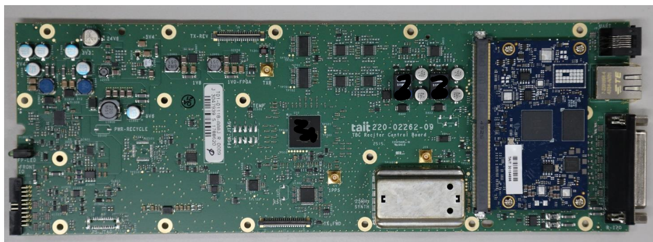
Photograph 05: Reciter Control board PCB – Top
