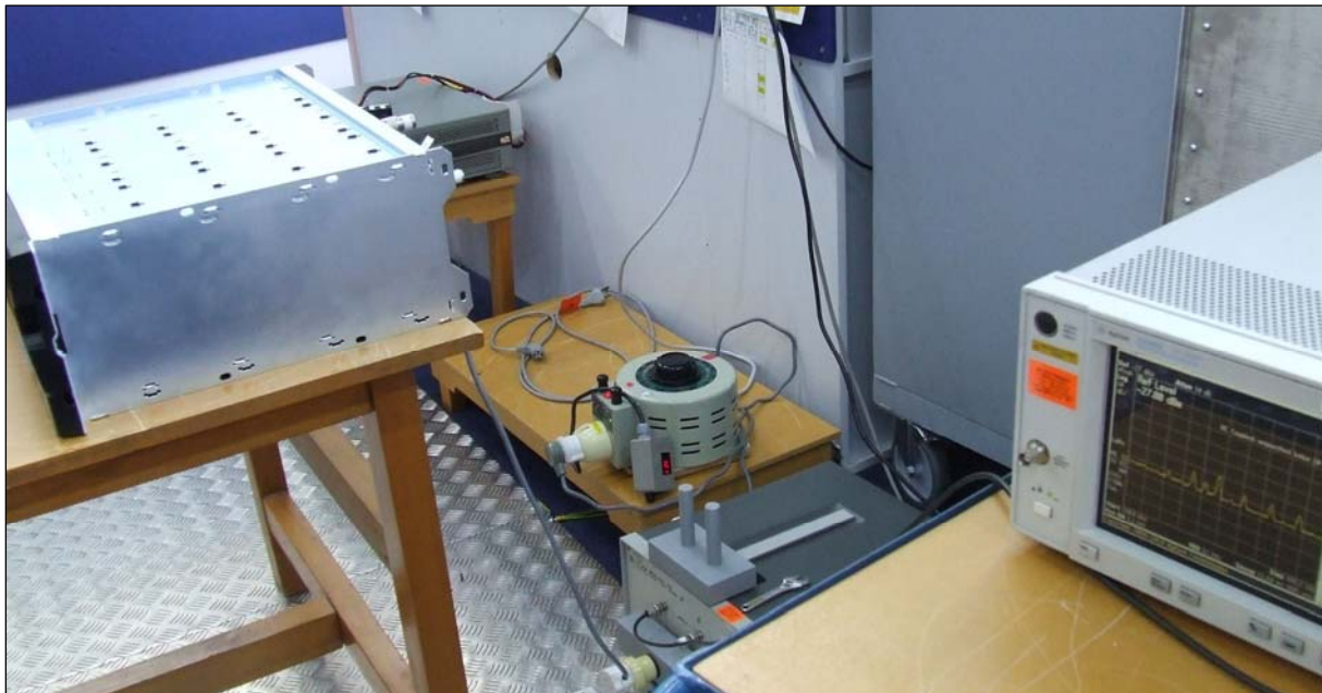
Photo: Power Line Conducted Emissions Setup
