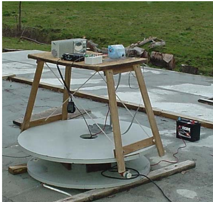
Radiated emissions test set up
