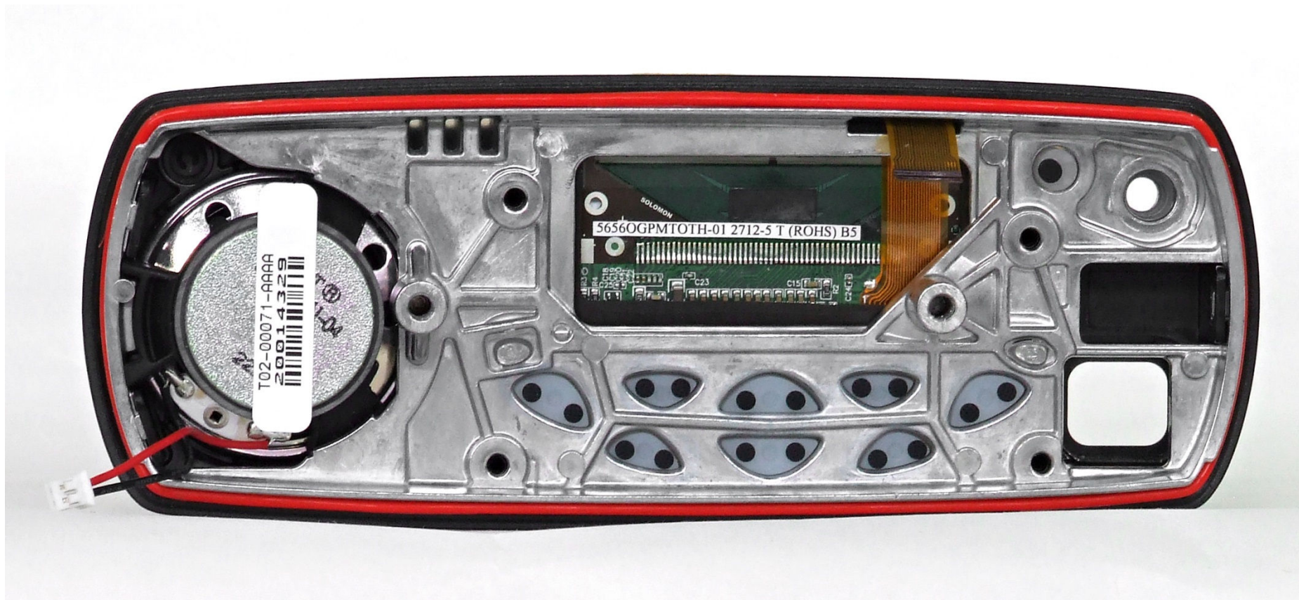
Photograph 08: Control Head – Internal with main PCB removed
