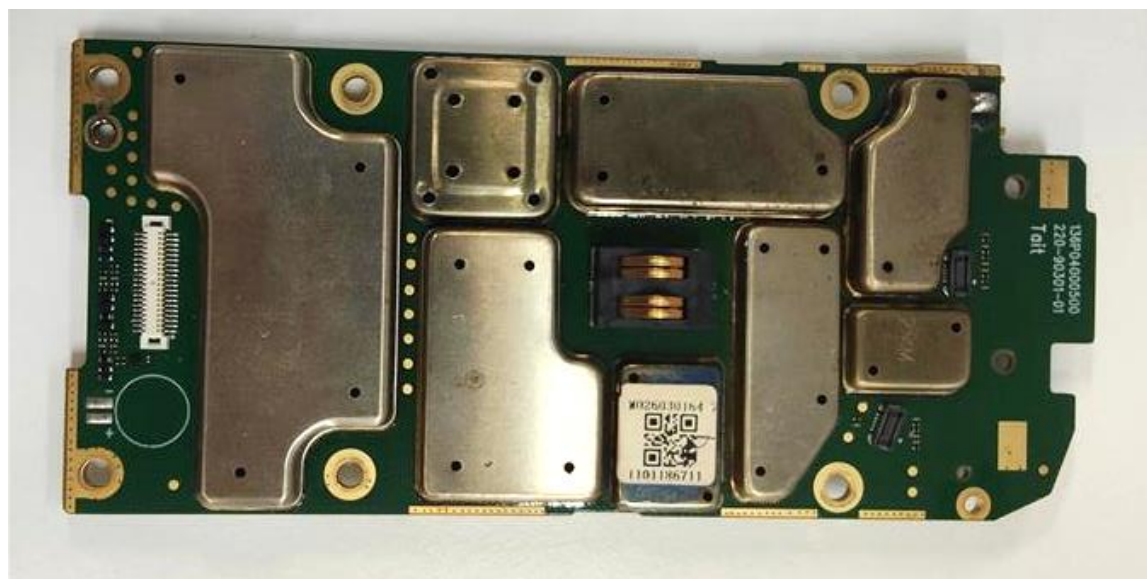
Photograph 01: Receive-Transmit PCB – top (with shields)
