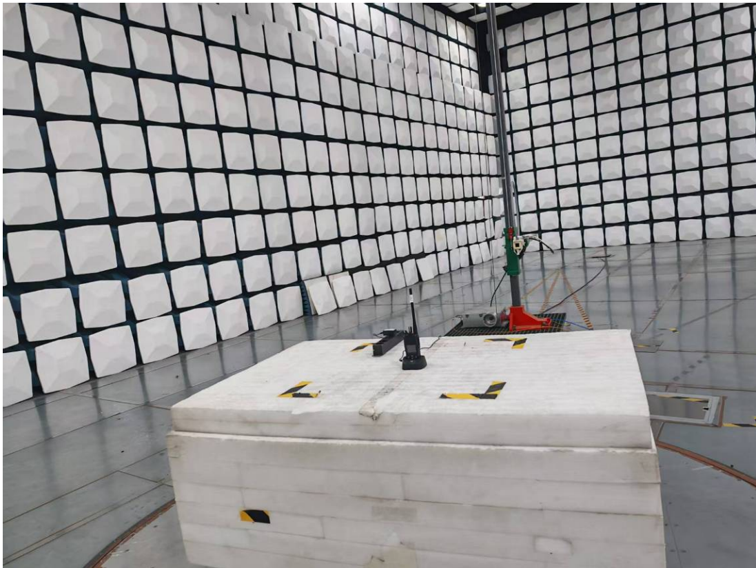
Radiated Emission 9k-30MHz Perpendicular View
