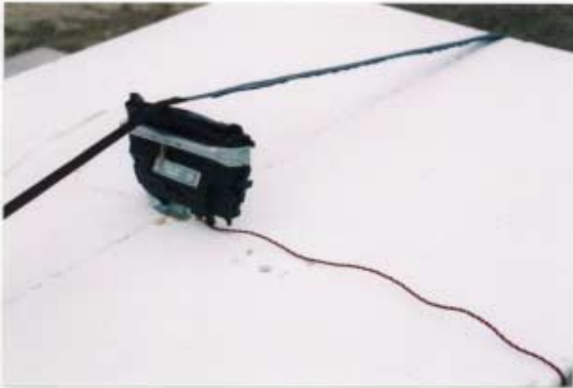
Appendix: Photos of the transmitter on the test table (Open-Site); the transmitter is tested when placed flat, on its side, and on its end. (top) Overall view, (bottom) Close-up.
