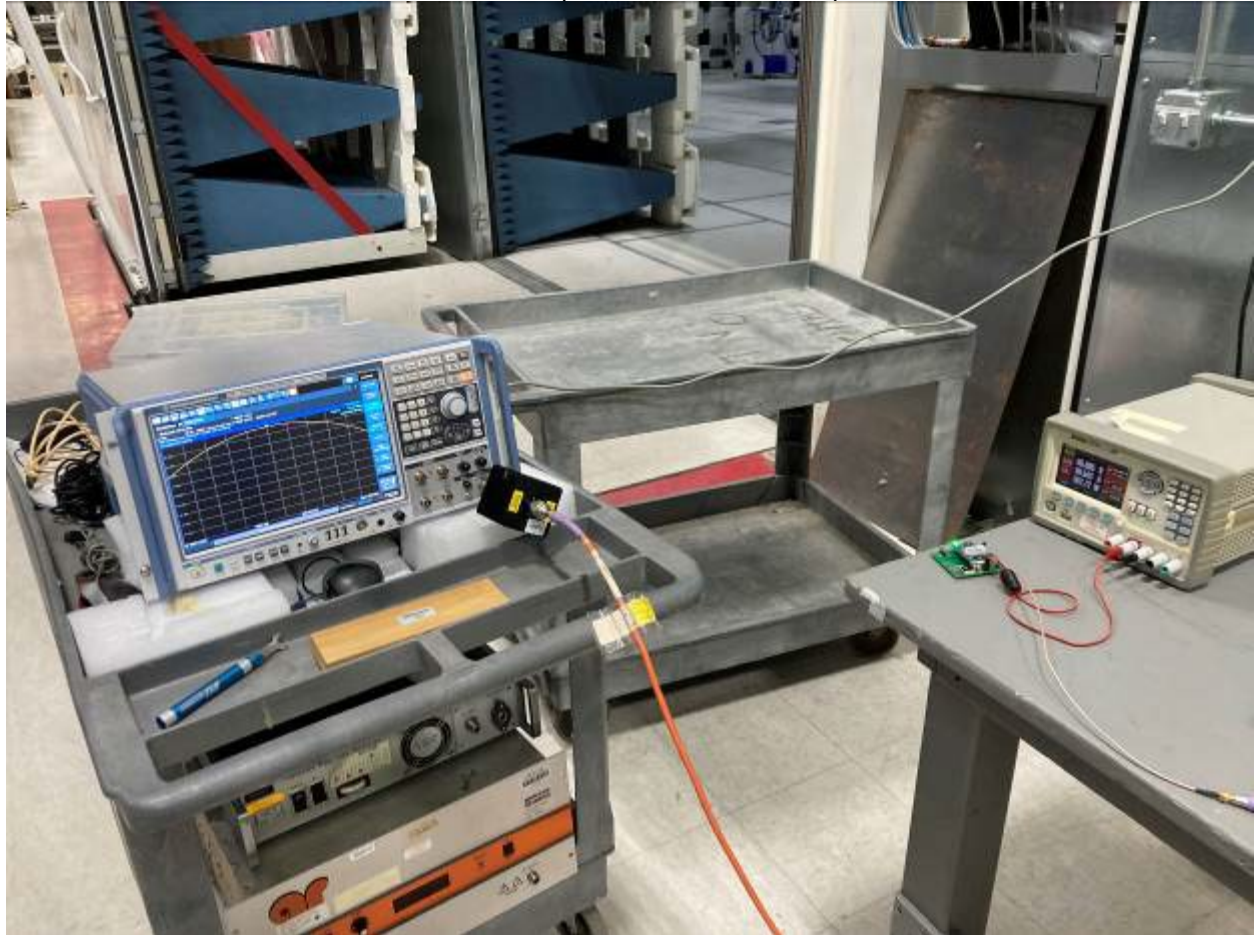
Conducted spurious emissions setup
