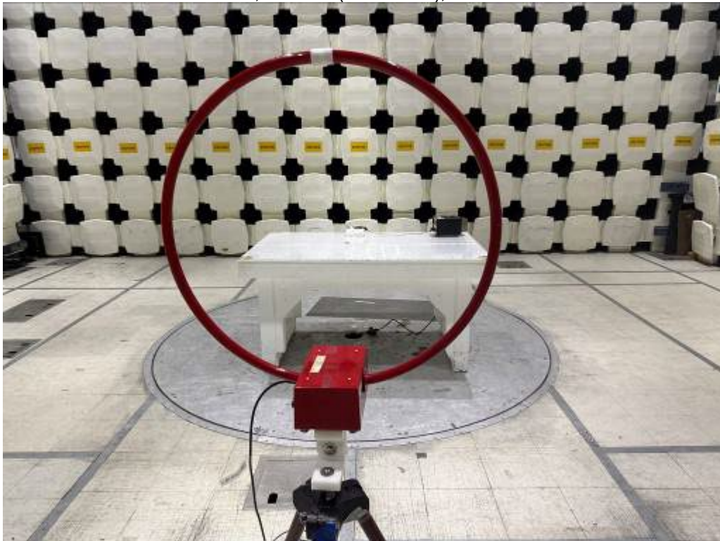
9 kHz – 30 MHz, EUT flat (worst case), Antenna on X-Axis
