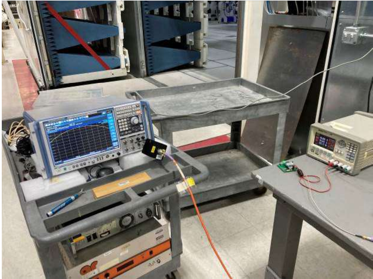
Antenna Port Conducted Output Power Measurements
