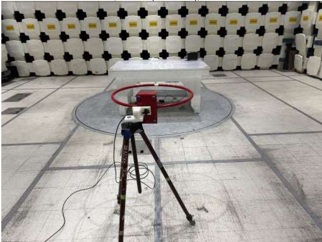
9 kHz – 30 MHz, EUT flat (worst case), Antenna on Z-Axis
