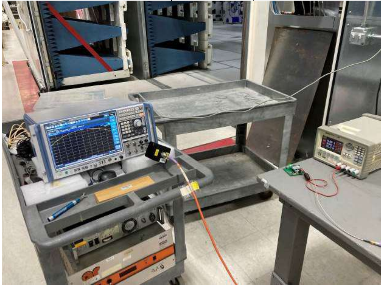
Conducted spurious emissions setup
