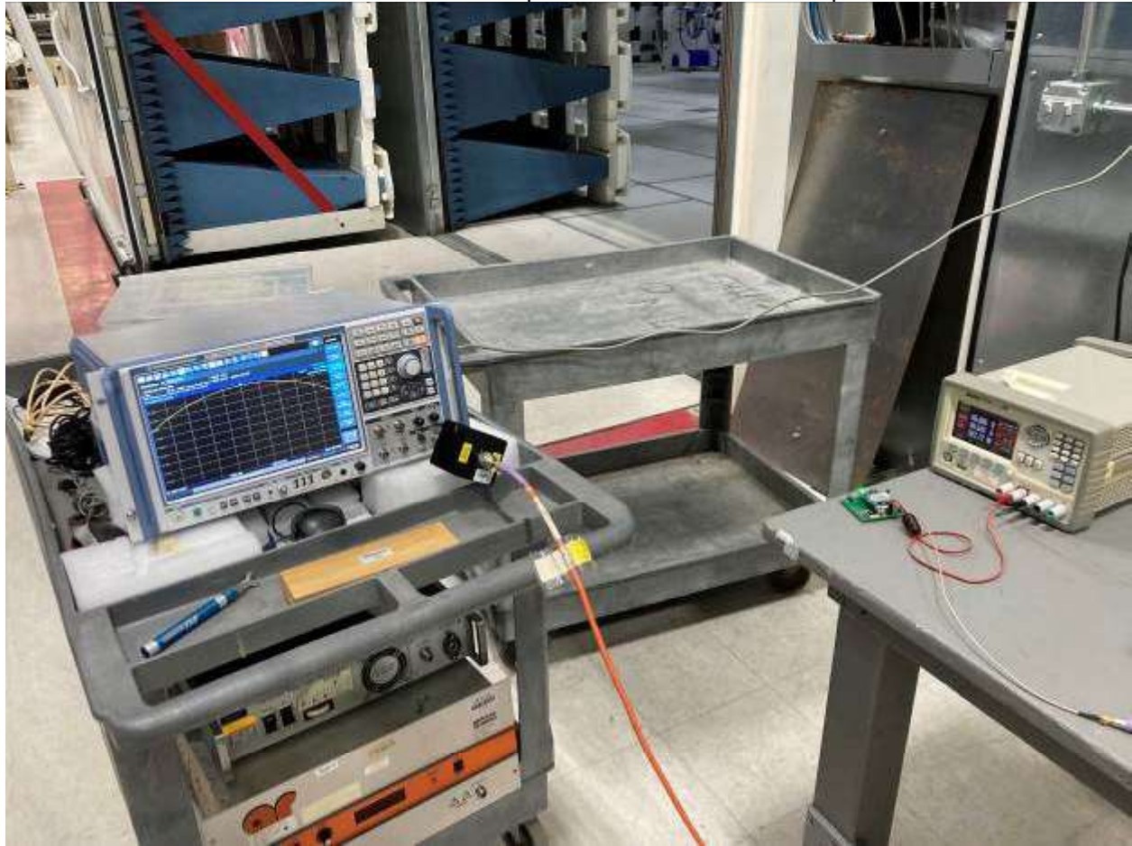
Antenna Conducted Spurious Emissions Test Setup
