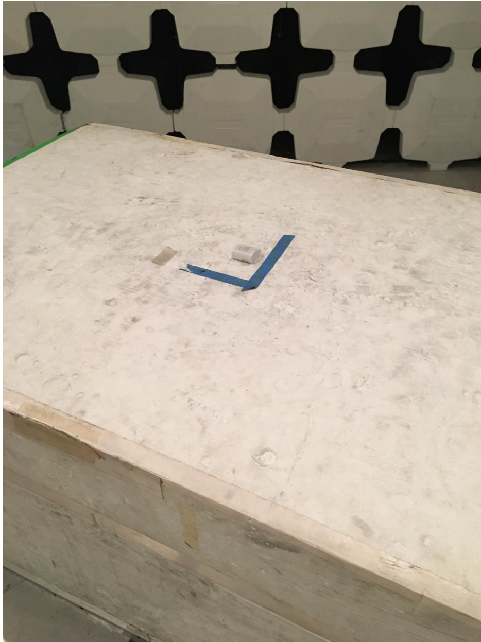
Figure 2. Radiated Emissions Test Setup 80 cm Test Height
