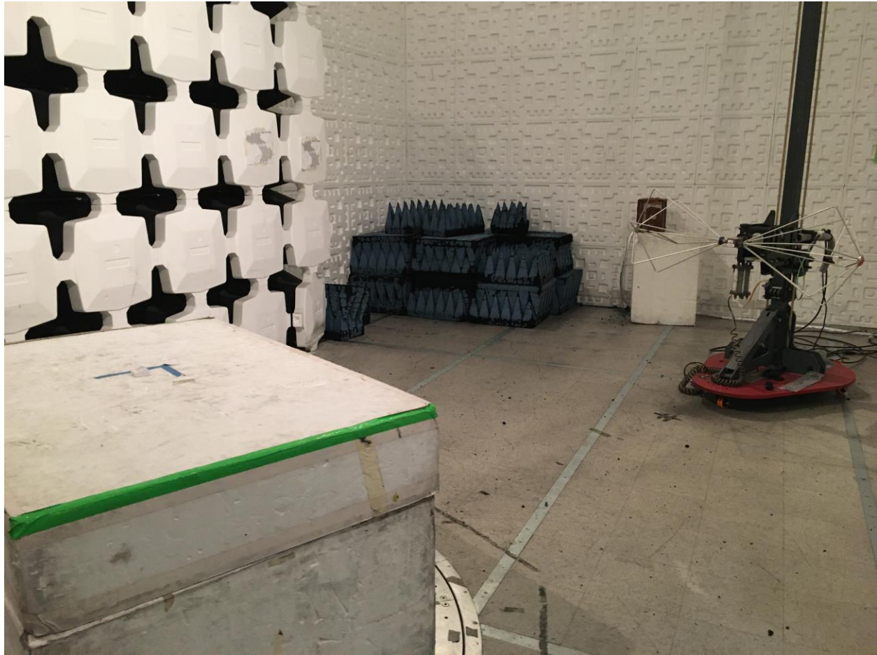
Figure 3. Radiated Emissions Test Setup, 30 to 200 MHz, Biconical Antenna
