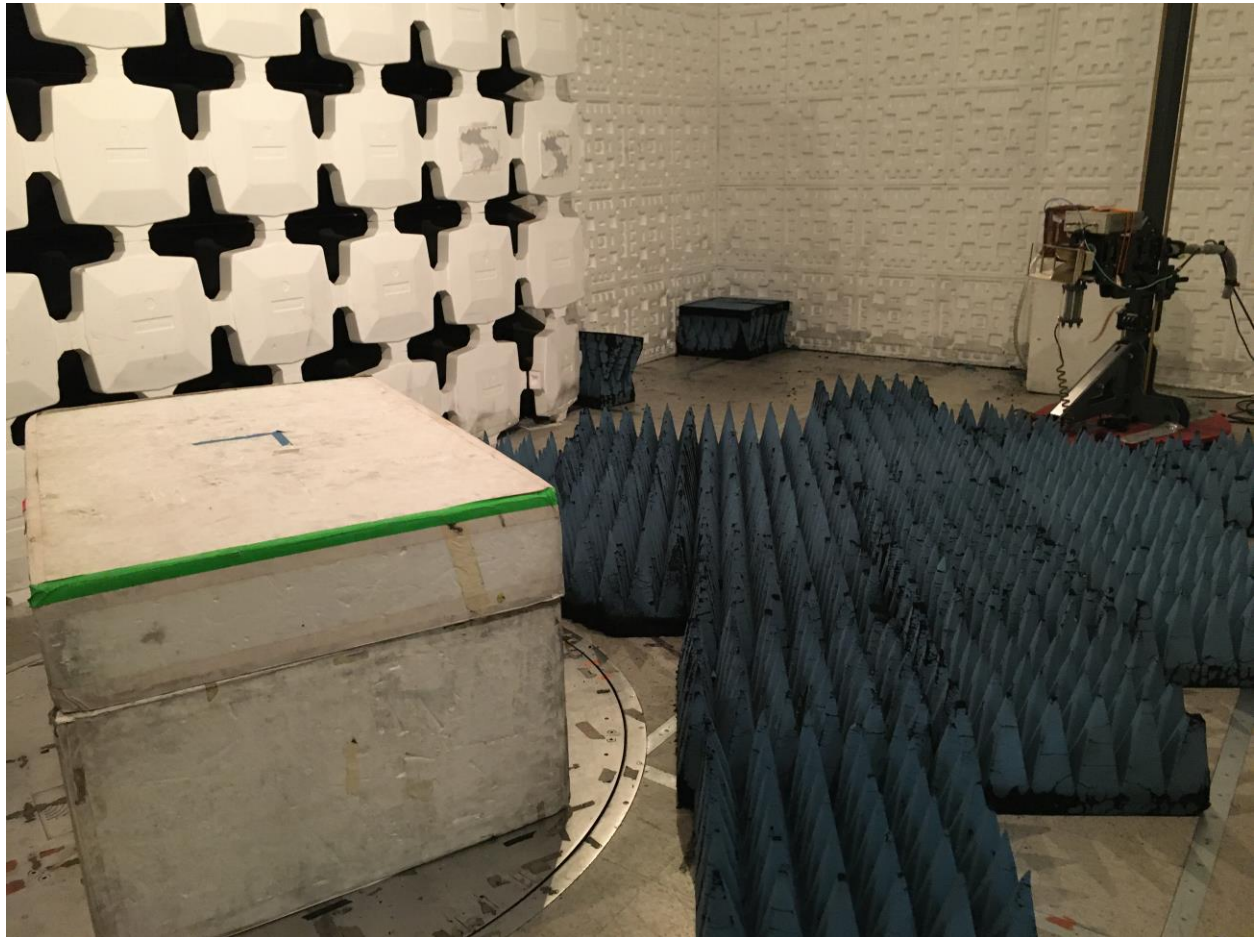
Figure 5. Radiated Emissions Test Setup, Above 1 GHz, Horn Antenna
