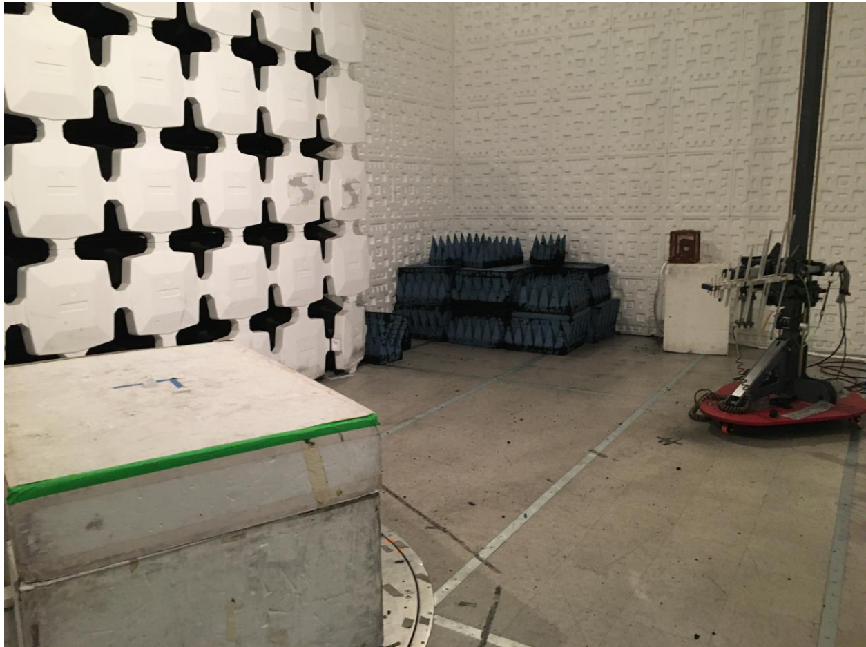
Figure 4. Radiated Emissions Test Setup, 200 to 1000 MHz, Log Periodic Antenna
