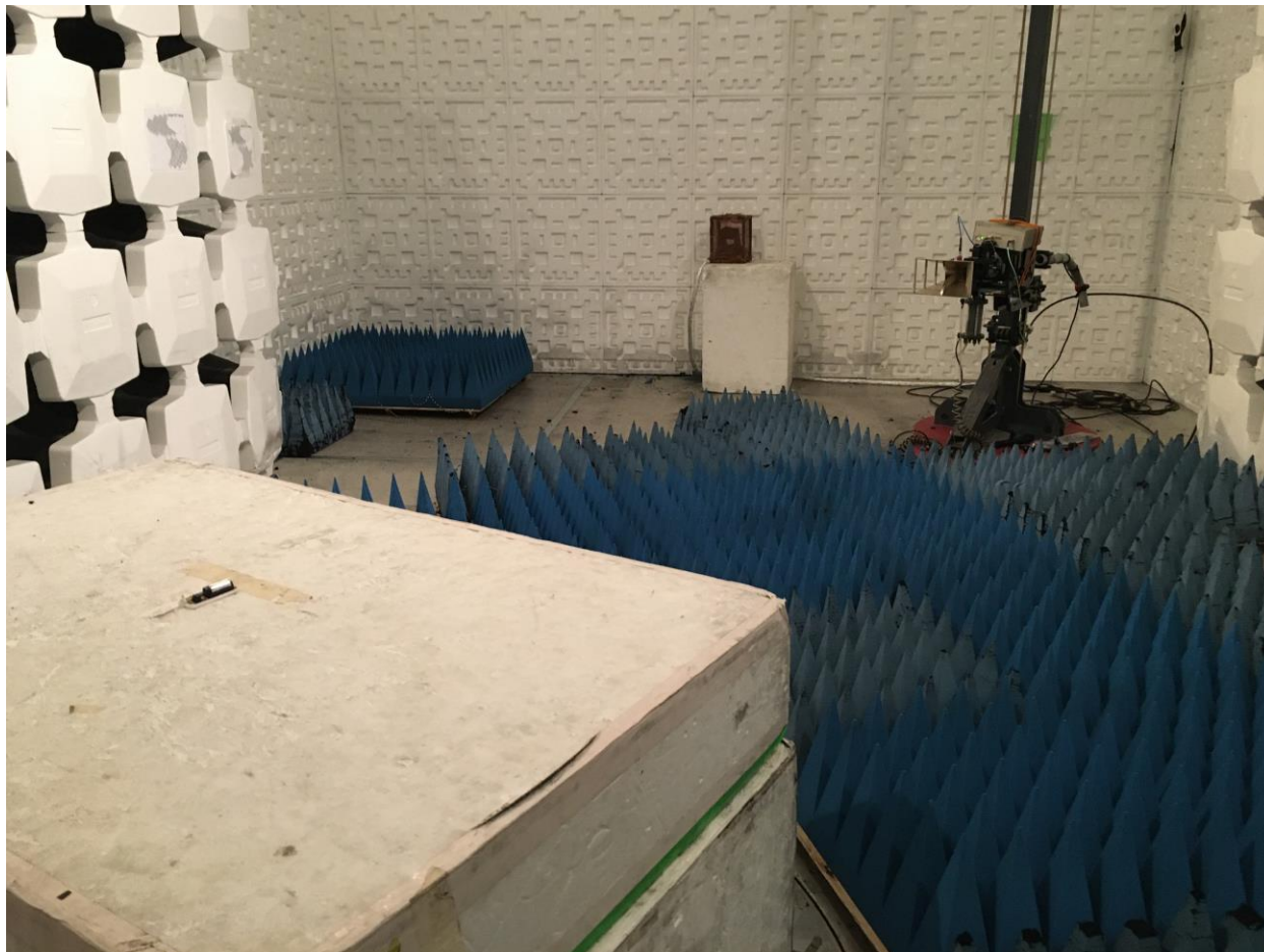
Figure 5. Radiated Emissions Test Setup, Above 1 GHz, Horn Antenna (80cm test height)
