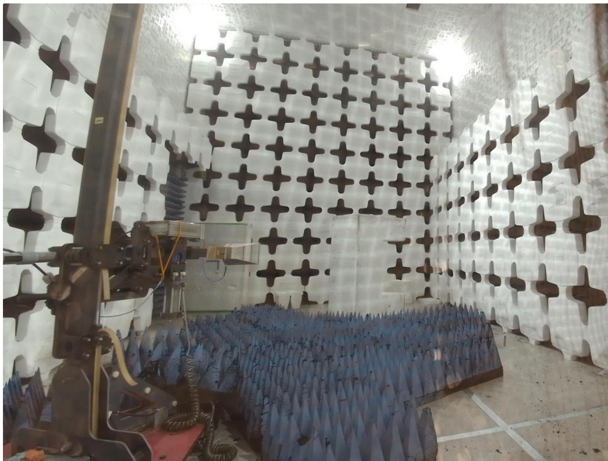
Figure 6. Radiated Emissions Test Setup, Above 1 GHz, Horn Antenna (150cm test height)
