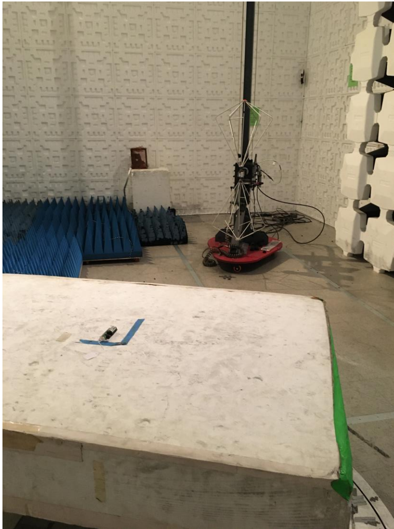
Figure 2. Radiated Emissions Test Setup 30 - 200 MHz
