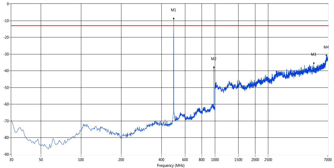
Figure 6: TX Spurious Radiation, 30 – 7000 MHz, Vertical (High CH)
