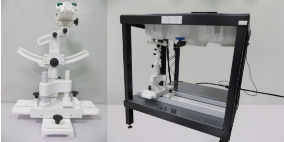
Device holder supplied by SATIMO
