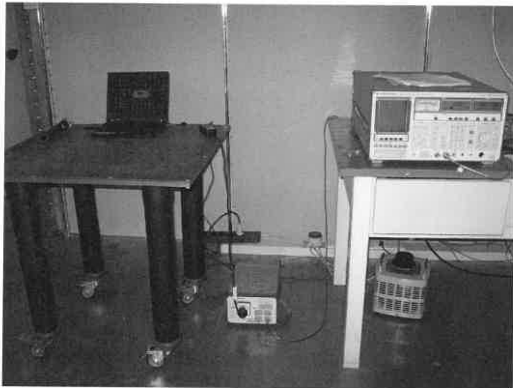
Photograph 1: Set-up for Conducted Emission
