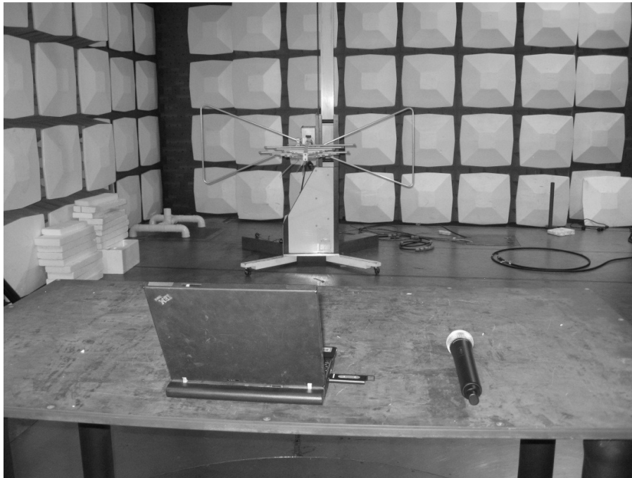
Photograph 2: Set-up for Radiated Emission (30MHz-1GHz)
