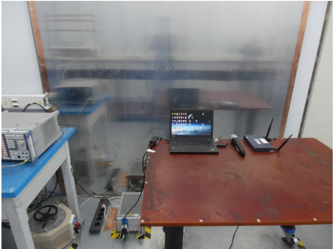
Photograph 1: Set-up for Conducted Emission
