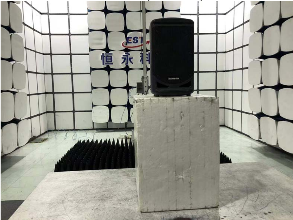
Radiated Test (Above 1GHz)
