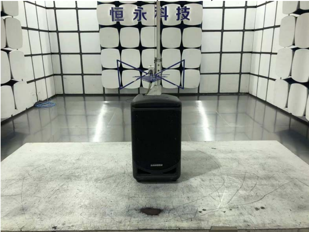
Radiated Test (Below 1GHz)
