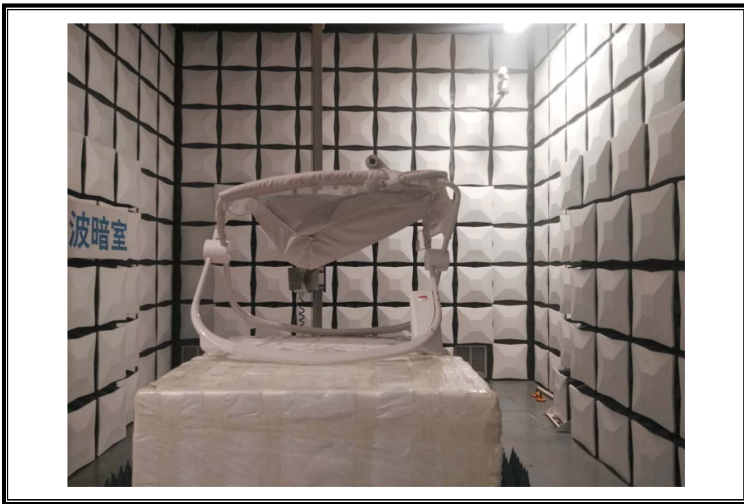
RADIATED RF MEASUREMENT SETUP (ABOVE 1 GHz)
