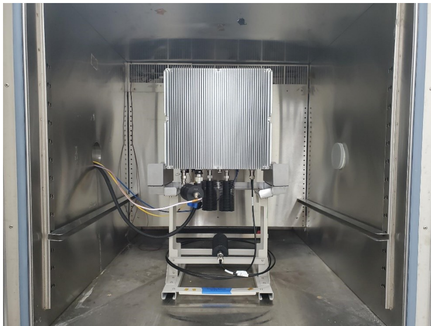
Figure 7 – Test setup – frequency stability measurements
