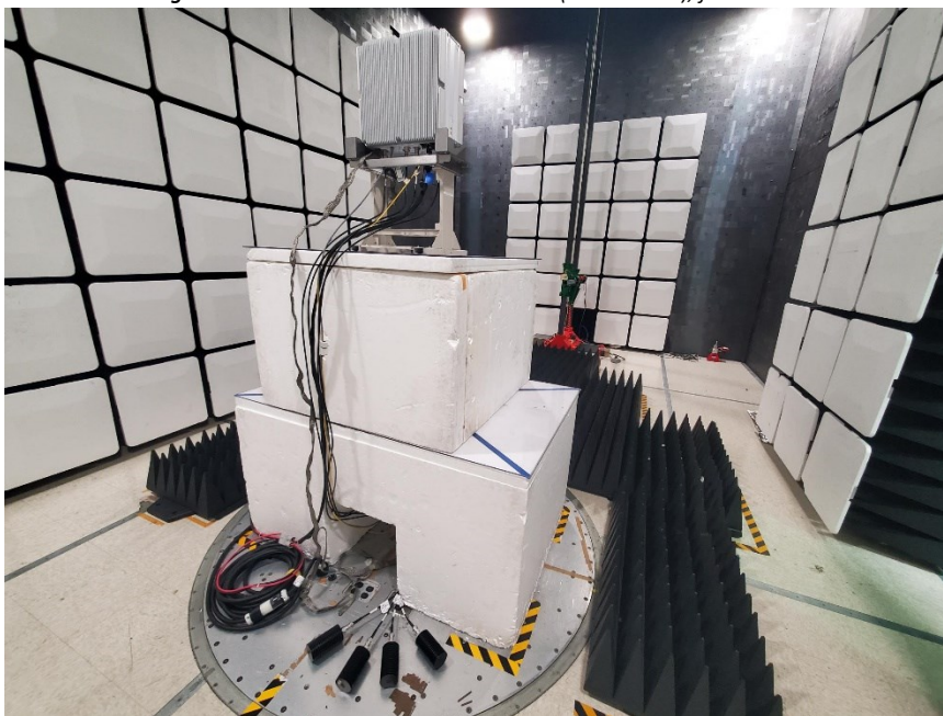
Figure 6 - Radiated emissions above 1 GHz (18 – 26 GHz), rear view.
