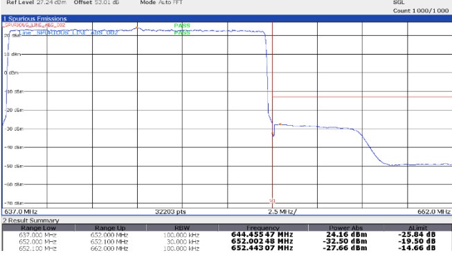
Band Edge. TX:644.5MHz, BW:15MHz, MOD: QPSK
