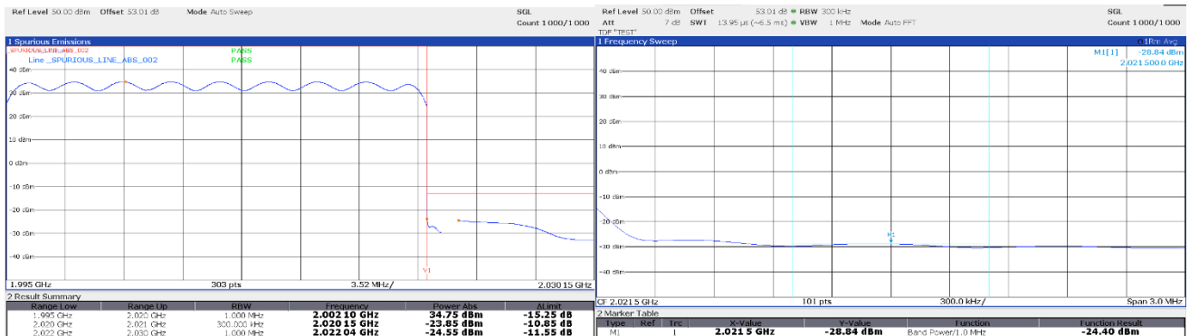
Band Edge. TX:2007.5MHz, BW:25MHz, MOD: 16QAM
