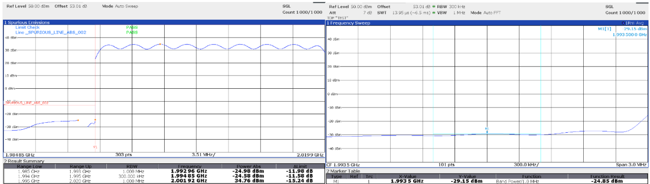
Band Edge. TX:2007.5MHz, BW:25MHz, MOD: 16QAM
