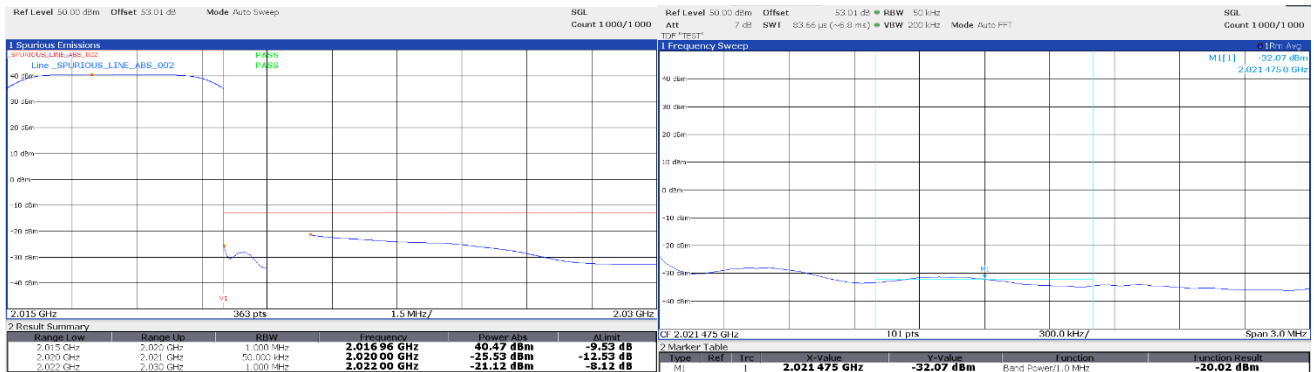
Band Edge. TX:2017.5MHz, BW:5MHz, MOD: 256QAM
