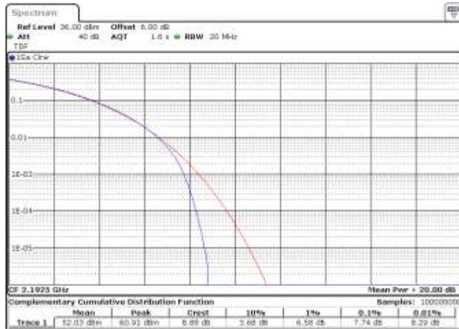
Figure 8.5-2: Peak to average power ratio, QPSK Modulation, high channel (15 MHz) and 16QAM Modulation, low channel (15 MHz), respectively, band n66.
