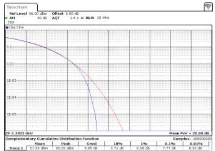
Figure 8.5-3: Peak to average power ratio, 16QAM Modulation, middle and high channel (15 MHz), respectively, band n66.
