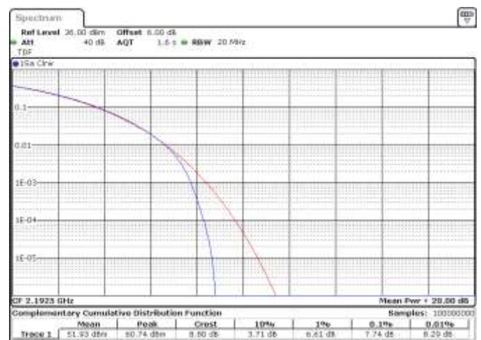
Figure 8.5-6: Peak to average power ratio, 256QAM Modulation, middle and high channel (15 MHz), respectively, band n66.
