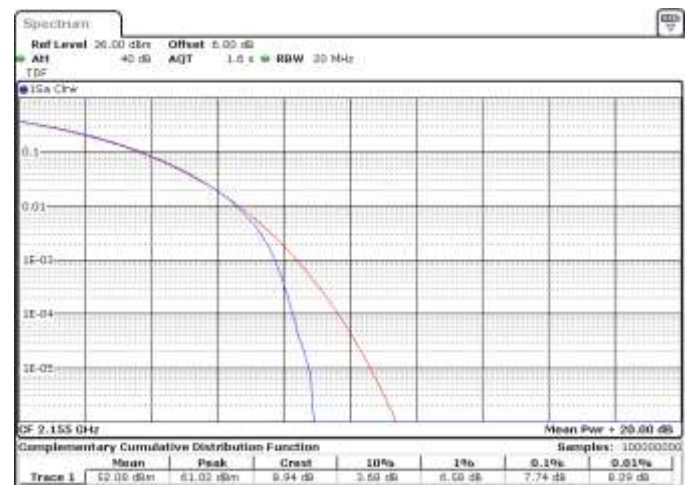
Figure 8.5-4: Peak to average power ratio, 64QAM Modulation, low and middle channel (15 MHz), respectively, band n66.
