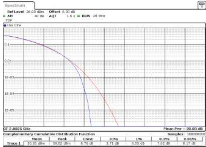
Figure 8.5-10: Peak to average power ratio, 256QAM Modulation, low and high channel (15 MHz), respectively, band n70.
