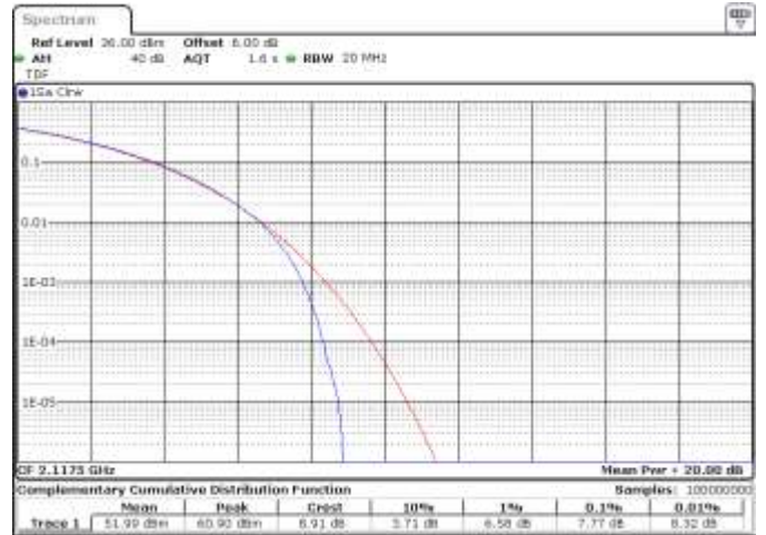
Figure 8.5-2: Peak to average power ratio, QPSK Modulation, high channel (15 MHz) and 16QAM Modulation, low channel (15 MHz), respectively, band n66.
