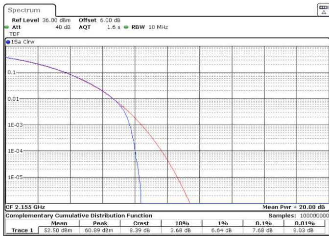
Figure 8.5-3: Peak to average power ratio, QPSK Modulation, middle and high channel (10 MHz), respectively, band n66.
