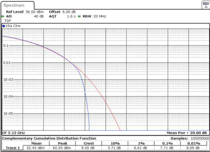
Figure 8.5-4: Peak to average power ratio, QPSK Modulation, low and middle channel (20 MHz), respectively, band n66.
