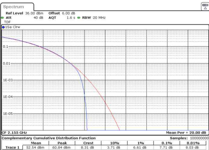
Figure 8.5-4: Peak to average power ratio, QPSK Modulation, low and middle channel (20 MHz), respectively, band n66.
