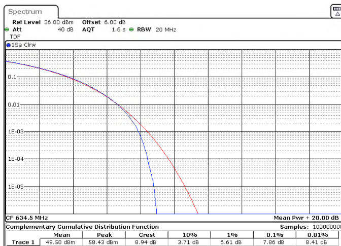
Figure 8.5-3: Peak to average power ratio, 16QAM, Modulation, middle channel (15 MHz) and high channel (15 MHz), respectively.
