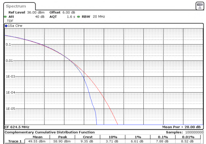
Figure 8.5-2: Peak to average power ratio, QPSK Modulation, high channel (15 MHz) and 16QAM Modulation, low channel (15 MHz), respectively.
