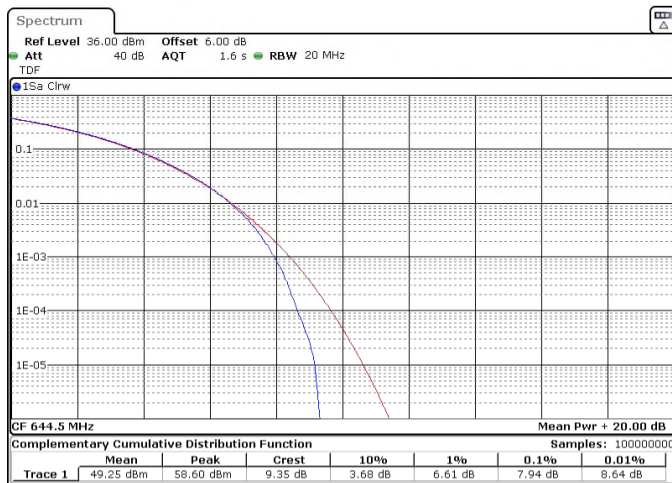
Figure 8.5-2: Peak to average power ratio, QPSK Modulation, high channel (15 MHz) and 16QAM Modulation, low channel (15 MHz), respectively.
