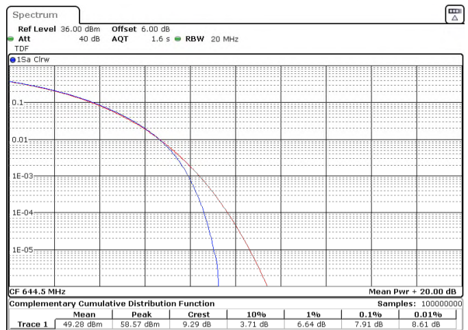
Figure 8.5-6: Peak to average power ratio, 256QAM, Modulation, middle channel (15 MHz) and high channel (15 MHz), respectively.
