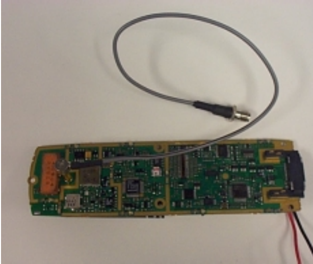
RF access port near antenna interface
