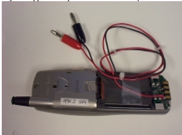
Fujitsu-supplied DC power connector interface mounted in the phone's battery compartment
