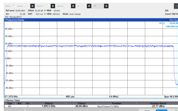
Figure 8.6-448: Conducted Spurious Emissions, High CH 1972.5 MHz, 45 MHz, QPSK, High band edge.
