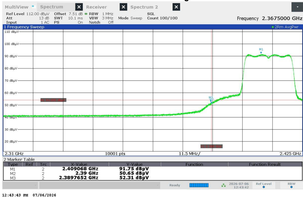
Figure 2.8.8.2-96 – Radiated Band Edge Emissions - Average
