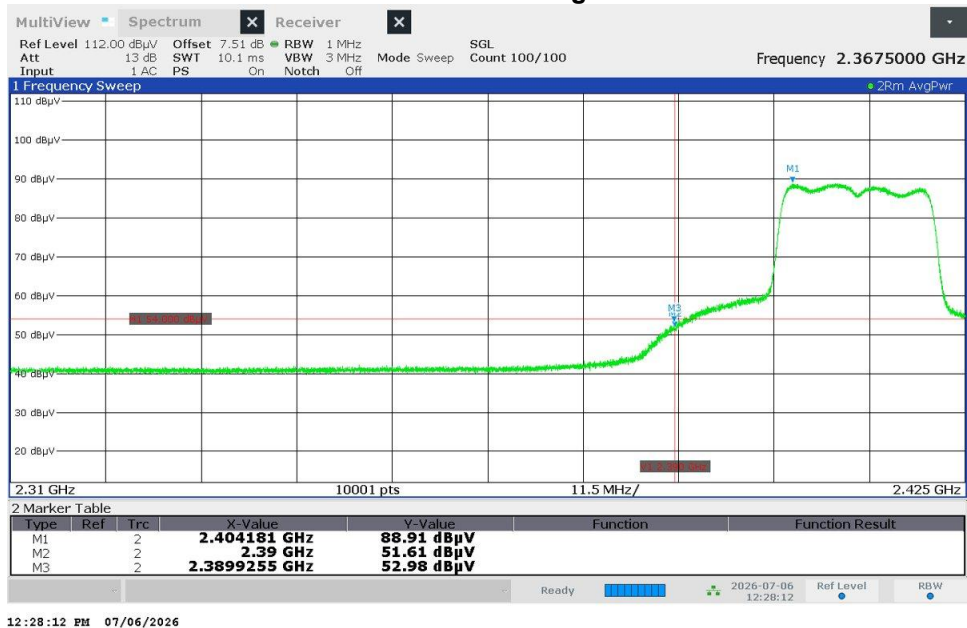
Figure 2.8.8.2-94 – Radiated Band Edge Emissions - Average
