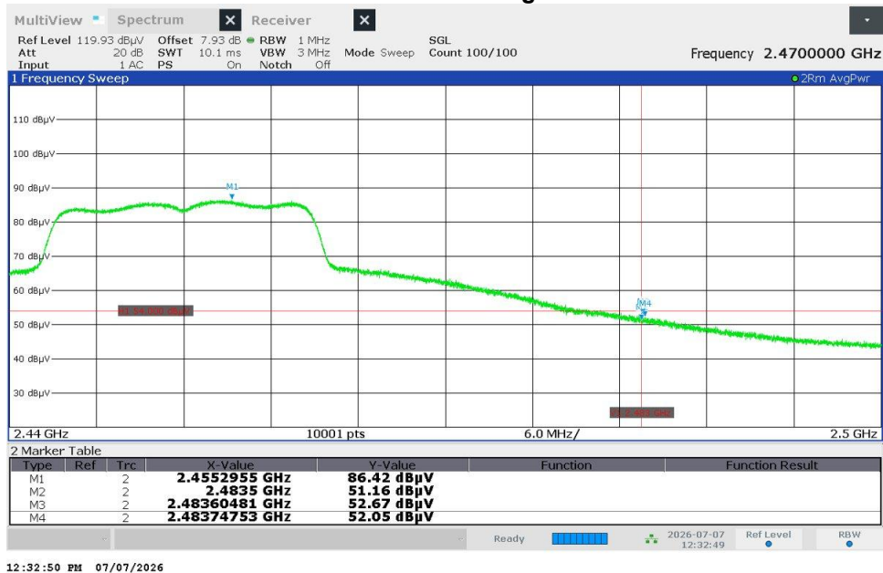
Figure 2.8.8.2-114 – Radiated Band Edge Emissions - Average
