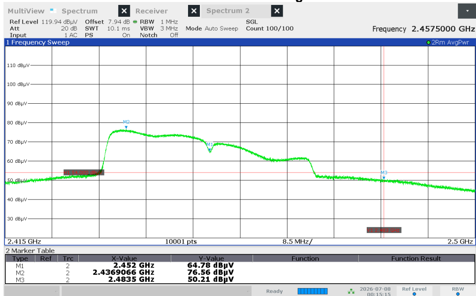
Figure 2.8.8.2-156 – Radiated Band Edge Emissions - Average
