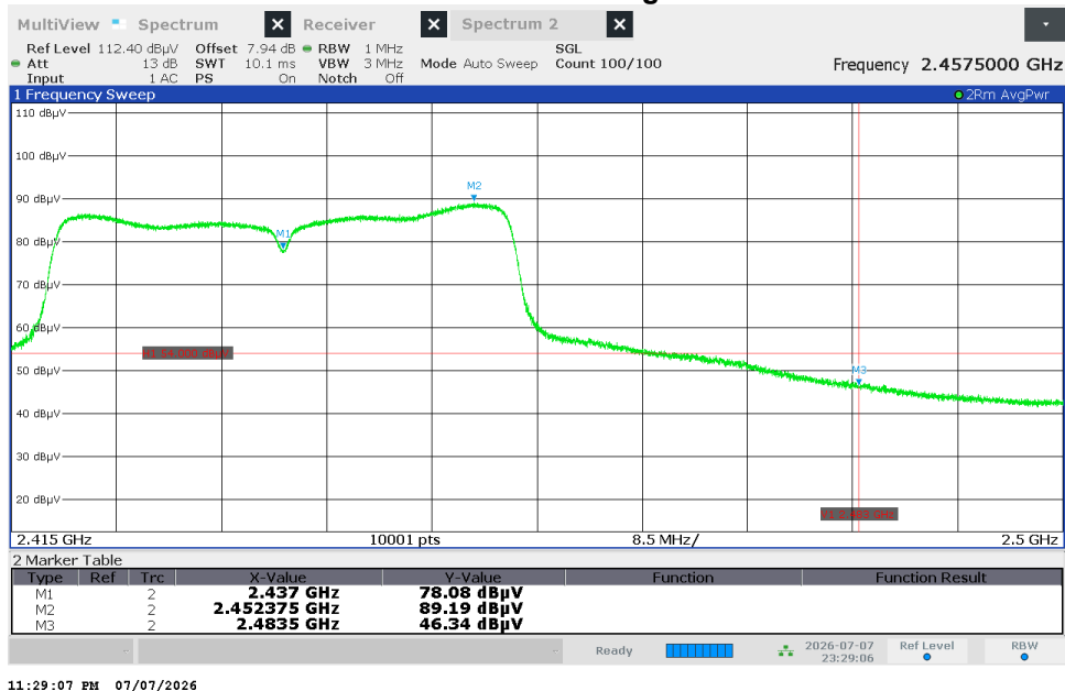
Figure 2.8.8.2-138 – Radiated Band Edge Emissions - Average
