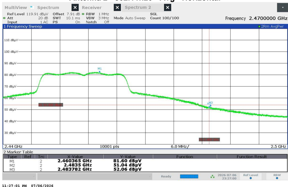
Figure 2.8.8.2-118 – Radiated Band Edge Emissions - Average
