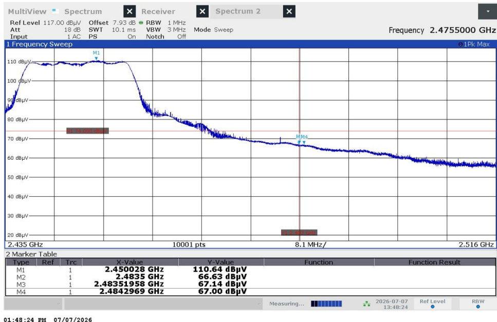
Figure 2.8.8.2-111 – Radiated Band Edge Emissions - Peak
