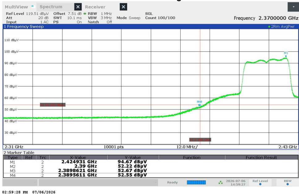
Figure 2.8.8.2-98 – Radiated Band Edge Emissions - Average
