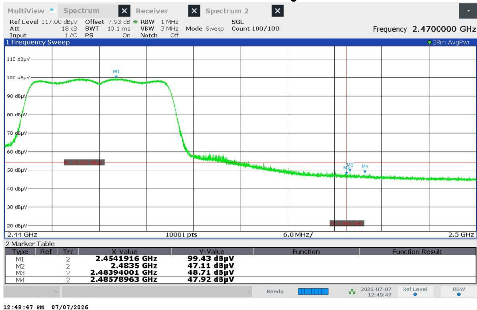
Figure 2.8.8.2-116 – Radiated Band Edge Emissions - Average
