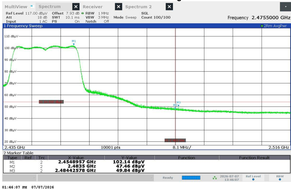
Figure 2.8.8.2-112 – Radiated Band Edge Emissions - Average
