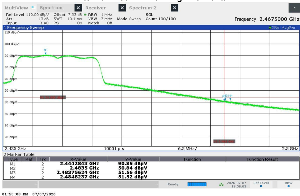
Figure 2.8.8.2-110 – Radiated Band Edge Emissions - Average
