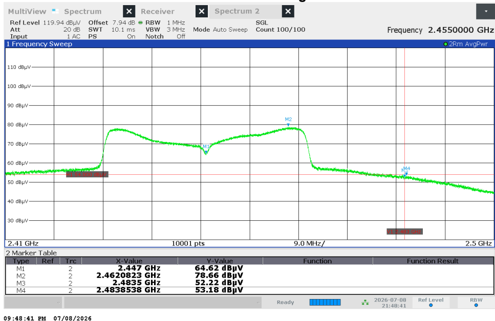
Figure 2.8.8.2-150 – Radiated Band Edge Emissions - Average
