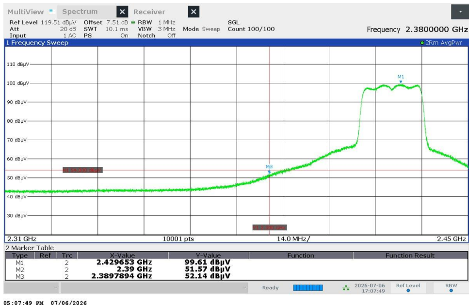
Figure 2.8.8.2-106 – Radiated Band Edge Emissions - Average
