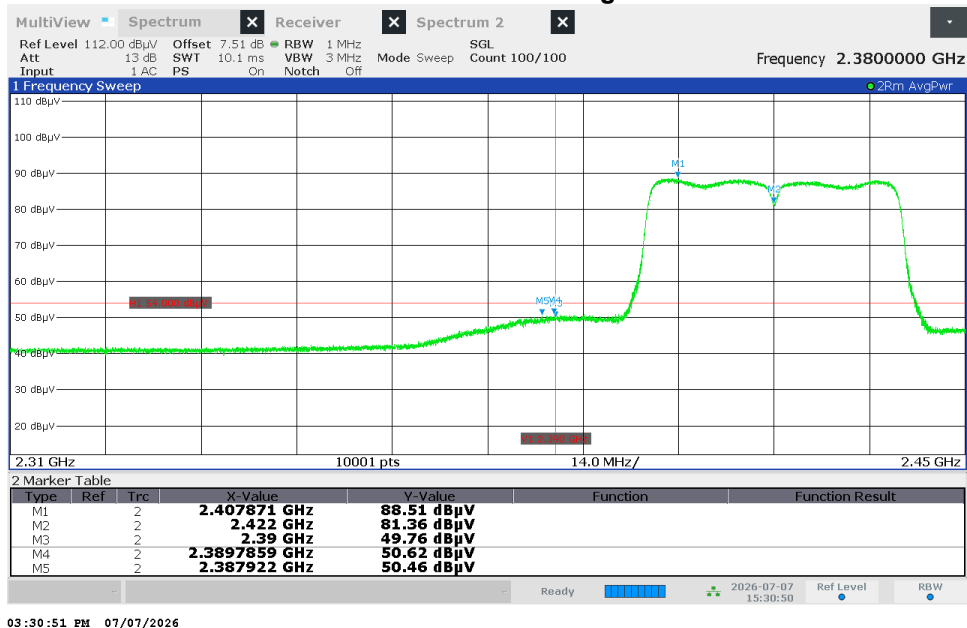
Figure 2.8.8.2-160 – Radiated Band Edge Emissions - Average
