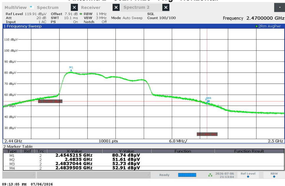
Figure 2.8.8.2-122 – Radiated Band Edge Emissions - Average
