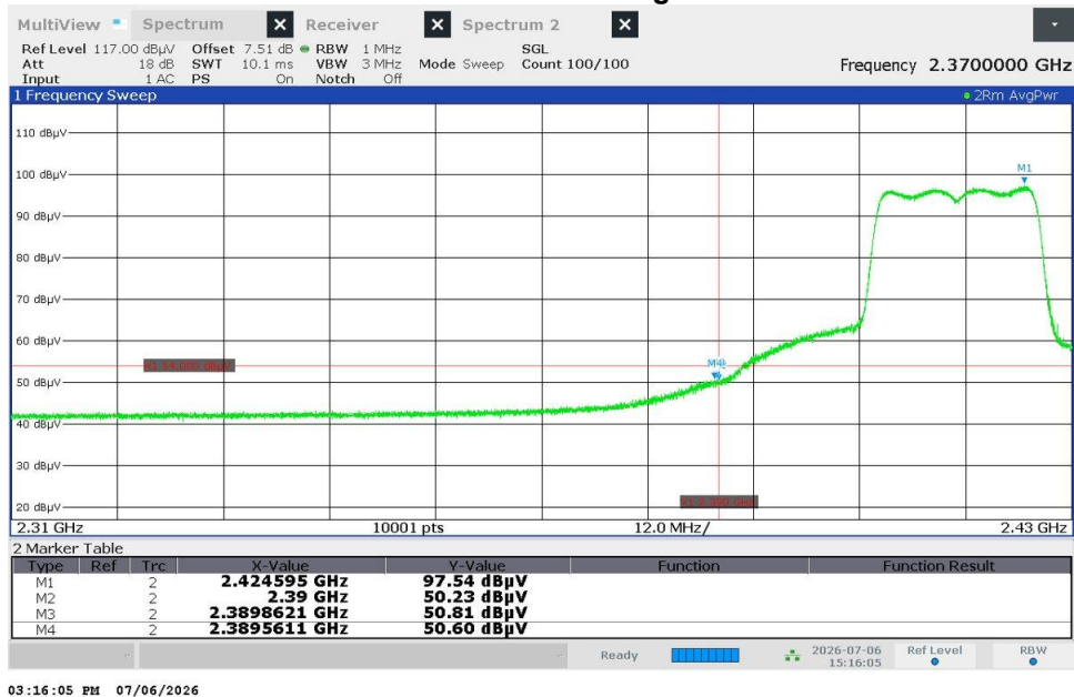
Figure 2.8.8.2-100 – Radiated Band Edge Emissions - Average
