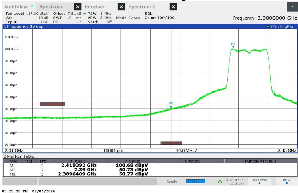
Figure 2.8.8.2-108 – Radiated Band Edge Emissions - Average
