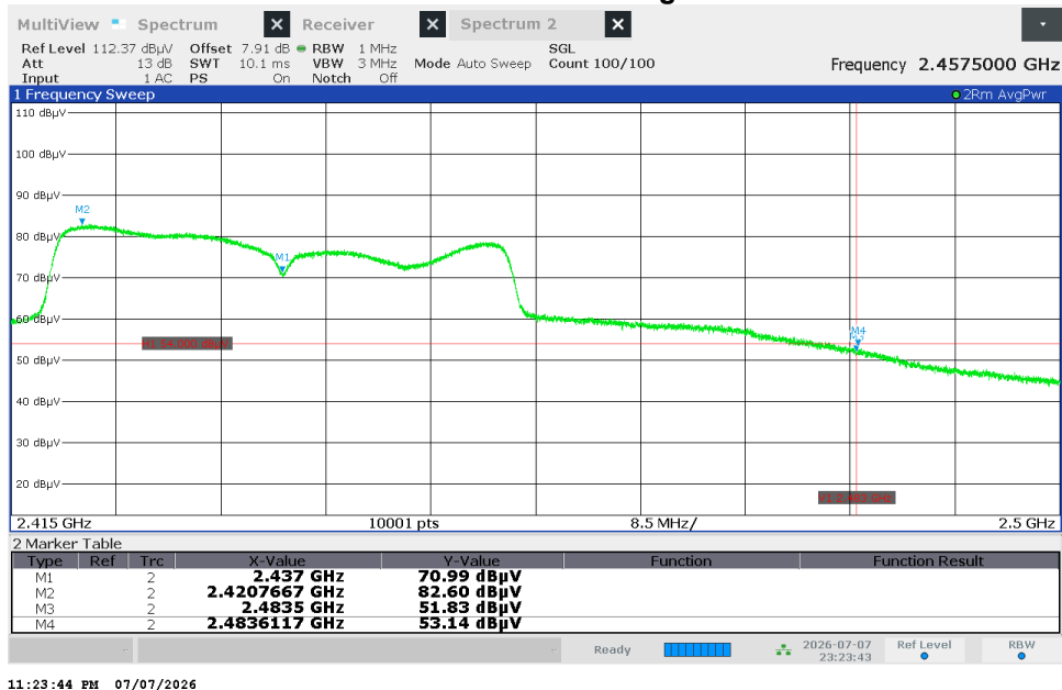
Figure 2.8.8.2-142 – Radiated Band Edge Emissions - Average
