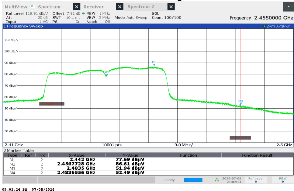
Figure 2.8.8.2-146 – Radiated Band Edge Emissions - Average
