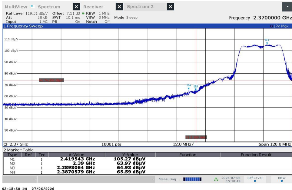
Figure 2.8.8.2-99 – Radiated Band Edge Emissions - Peak
