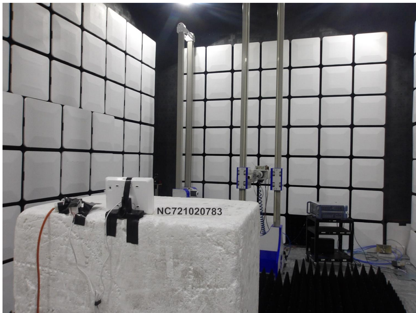
Photo 1-12 – Radiated Spurious Emissions 18GHz – 40GHz – Rear View
