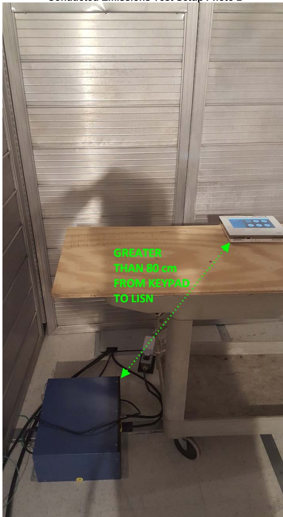
Conducted Emissions Test Setup Photo 2
