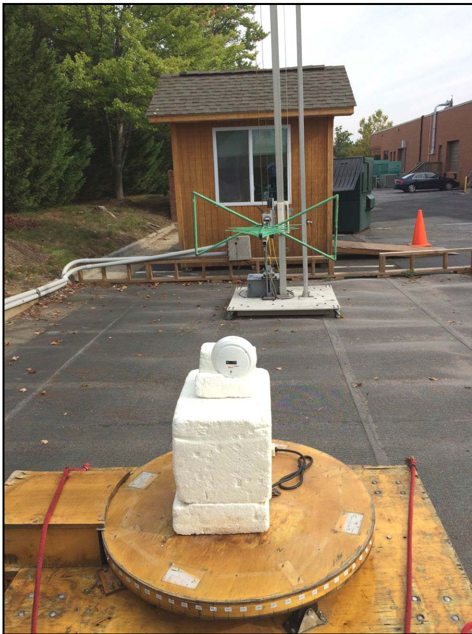
Photograph 1: Radiated Emissions Testing – Front View (Less than 1 GHz)
