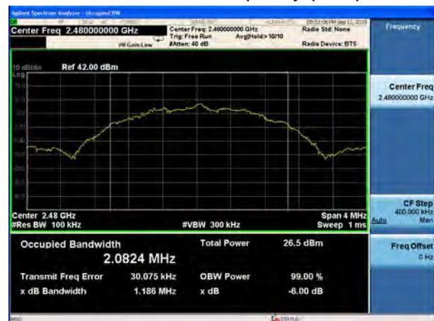
BLE V5.0-2M Carrier frequency (MHz): 2480
