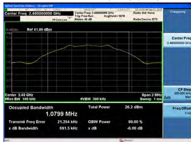
BLE V5.0-1M Carrier frequency (MHz): 2480
