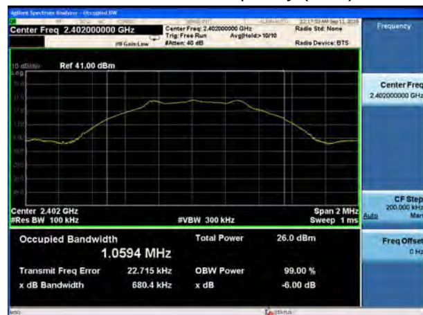
BLE V5.0-1M Carrier frequency (MHz): 2440
