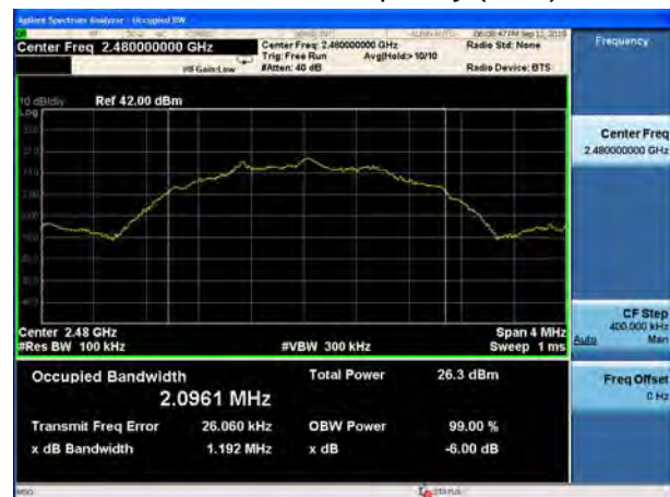
BLE V5.0-2M Carrier frequency (MHz): 2480
