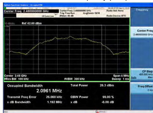
BLE V5.0-2M Carrier frequency (MHz): 2480
