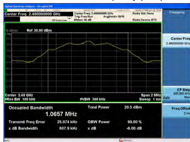
BLE V5.0-125K Carrier frequency (MHz): 2480
