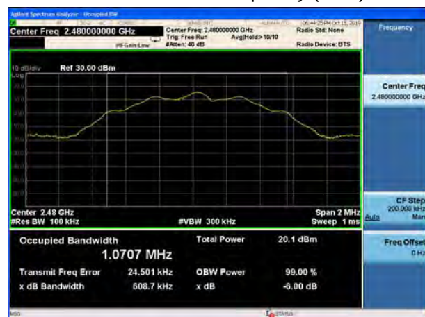
BLE V5.0-125K Carrier frequency (MHz): 2480
