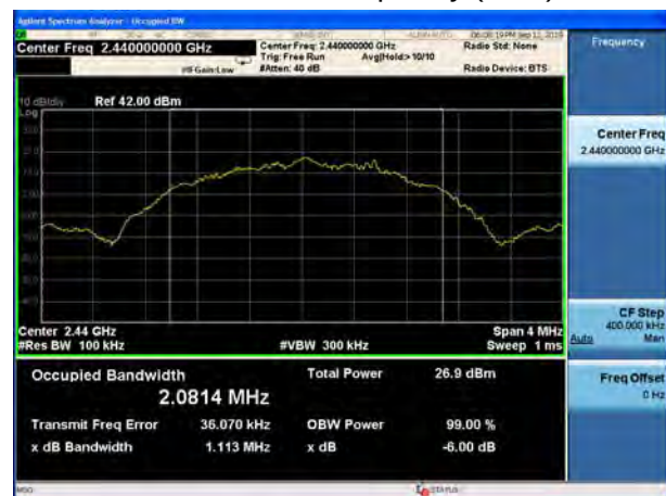
BLE V5.0-2M Carrier frequency (MHz): 2480
