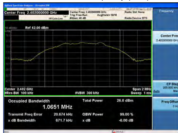
BLE V5.0-1M Carrier frequency (MHz): 2440
