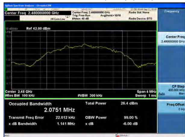
BLE V5.0-2M Carrier frequency (MHz): 2480
