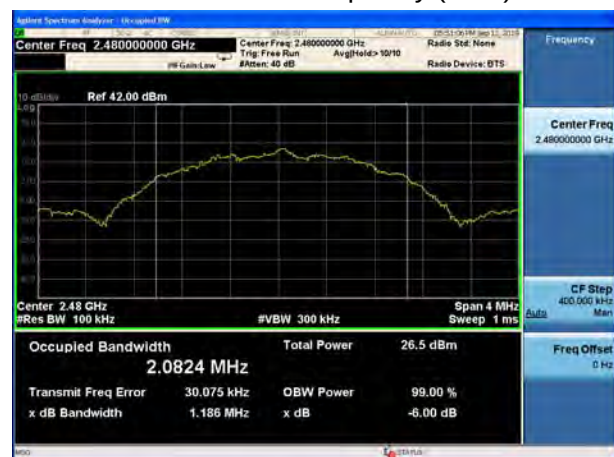
BLE V5.0-2M Carrier frequency (MHz): 2480
