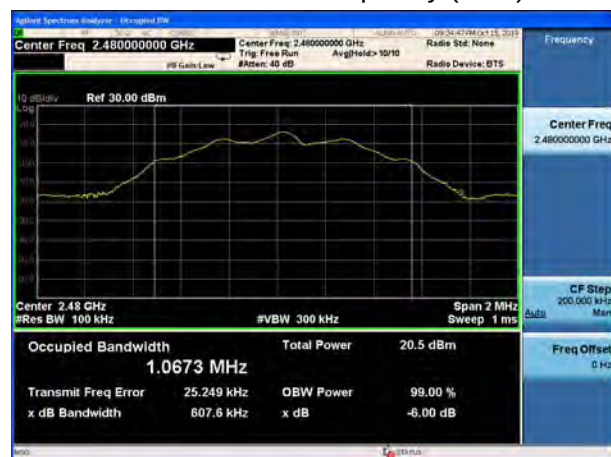
BLE V5.0-125K Carrier frequency (MHz): 2480
