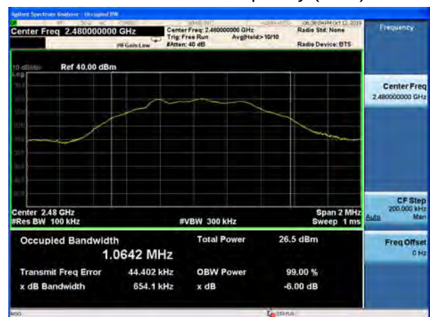
BLE V5.0-500K Carrier frequency (MHz): 2480
