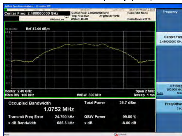
BLE V5.0-1M Carrier frequency (MHz): 2480
