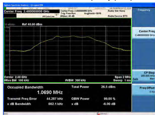
BLE V5.0-500K Carrier frequency (MHz): 2480
