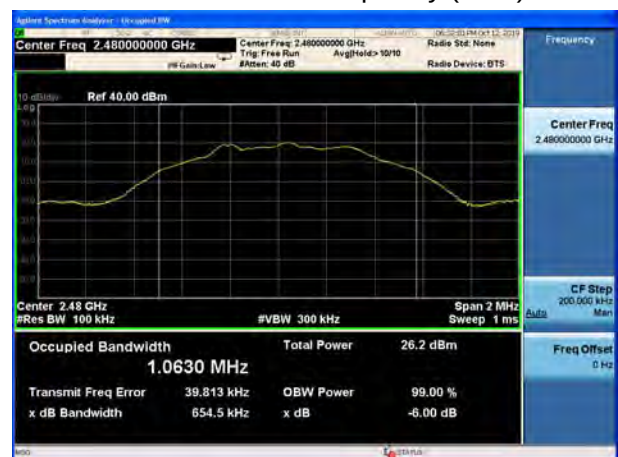
BLE V5.0-500K Carrier frequency (MHz): 2480
