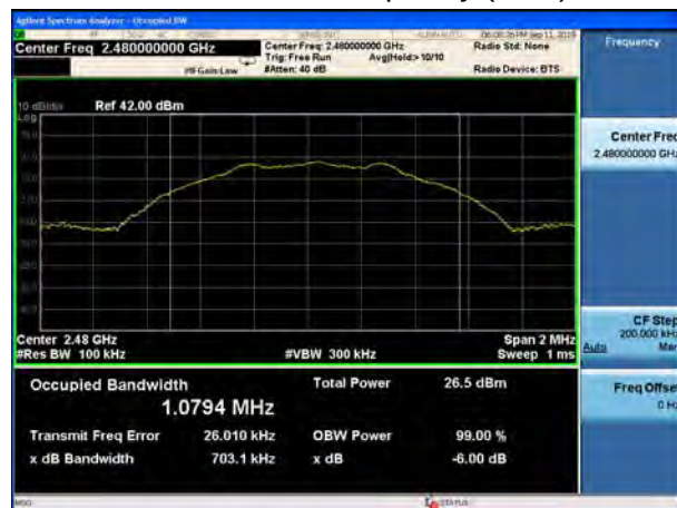
BLE V5.0-1M Carrier frequency (MHz): 2480
