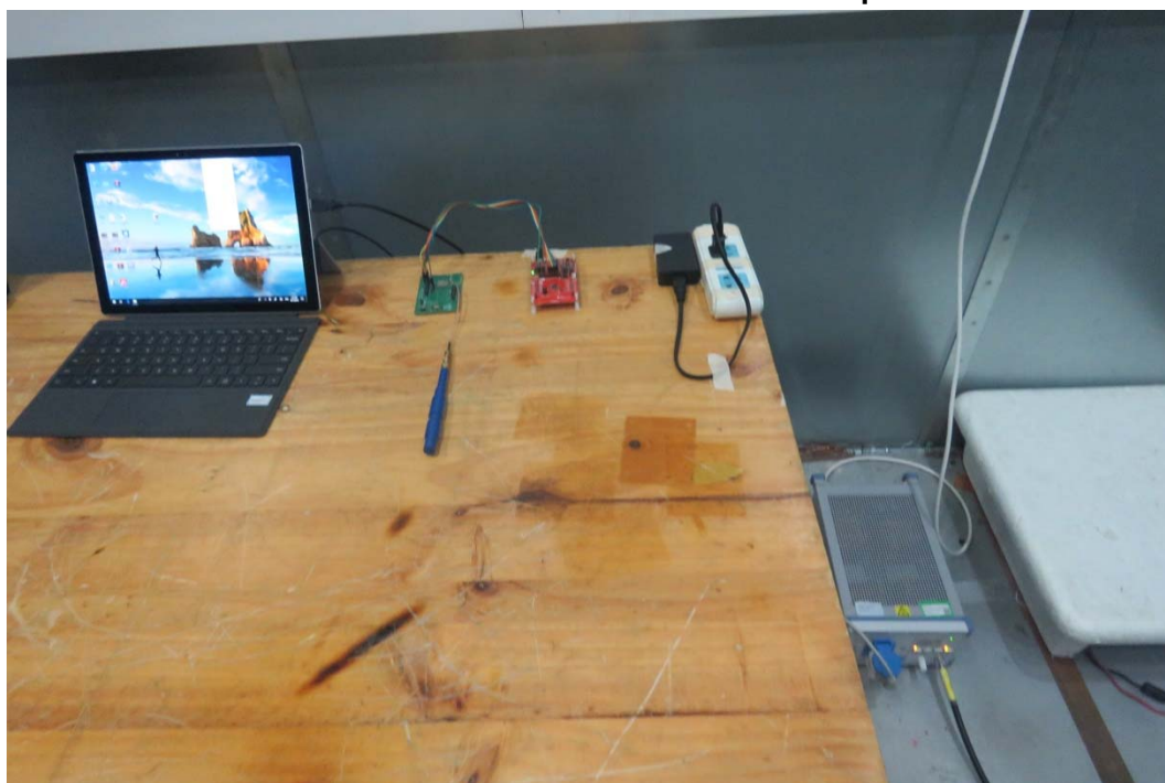
Picture 2 Conducted Emission Test Setup
