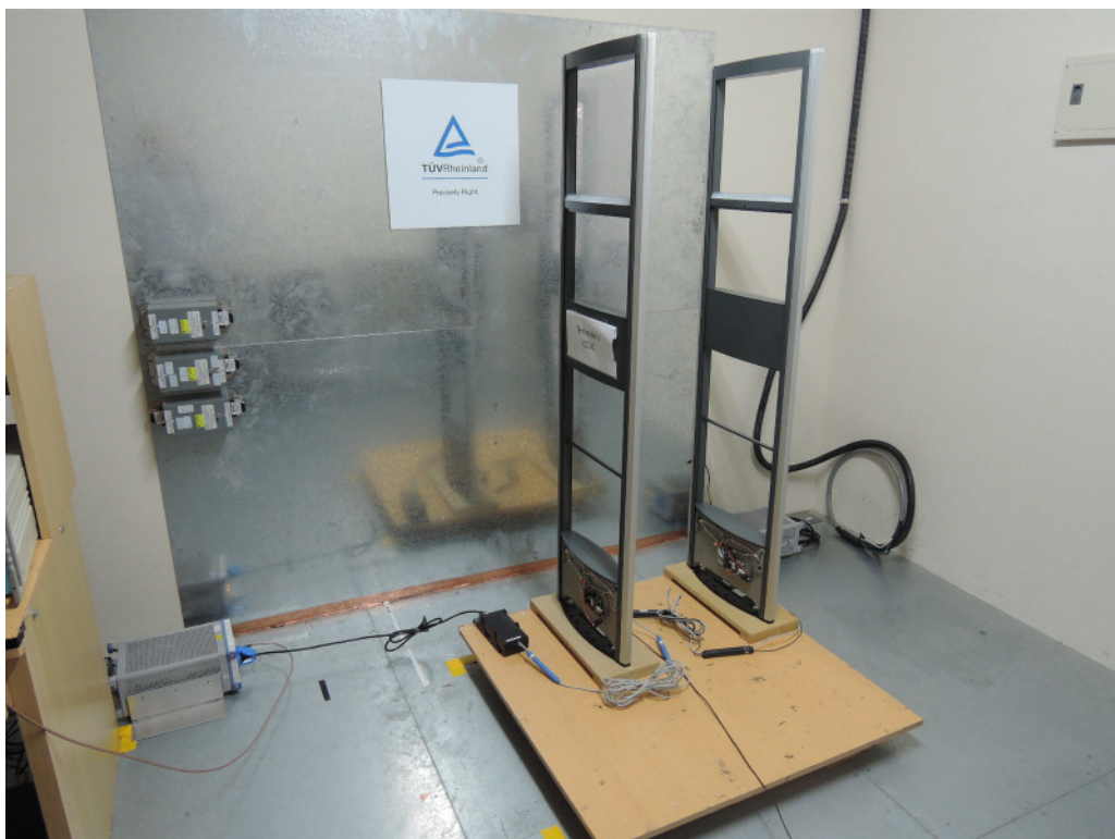
Photograph 5: Set-up for for Mains Conducted testing Front
