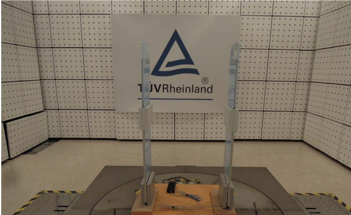
Photograph 1: Set-up for Radiated Emissions TX (Front View)
