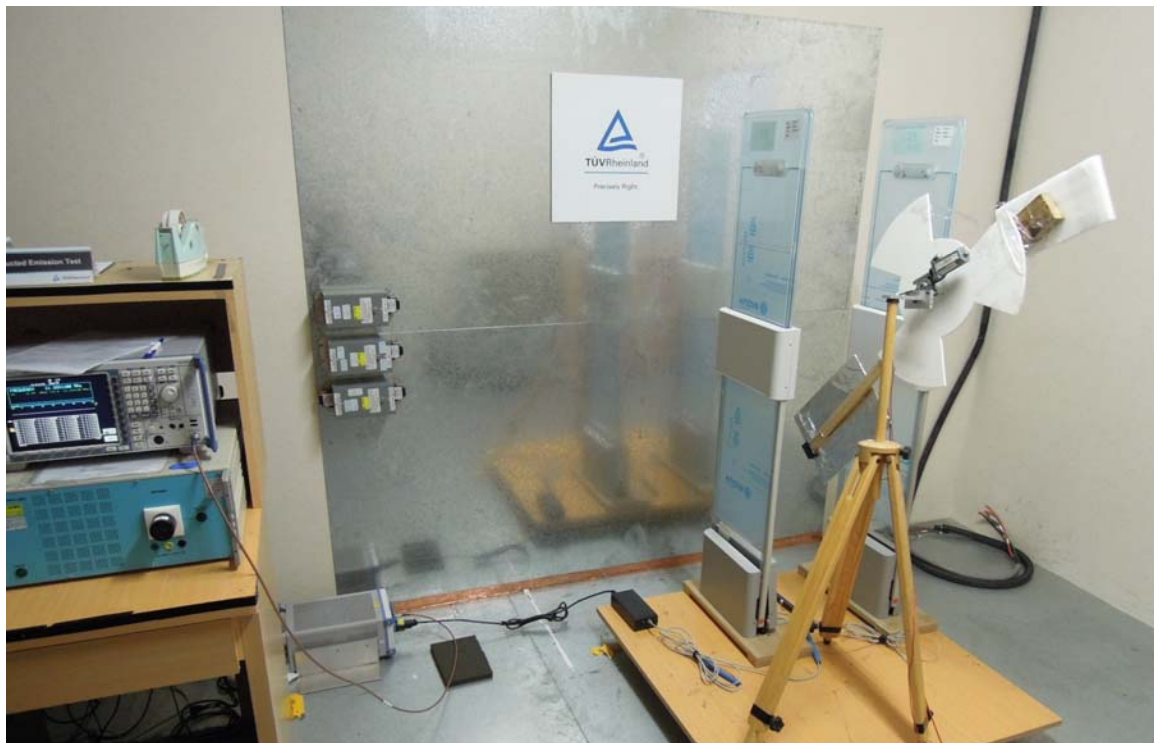
Photograph 5: Set-up for for Mains Conducted testing Front
