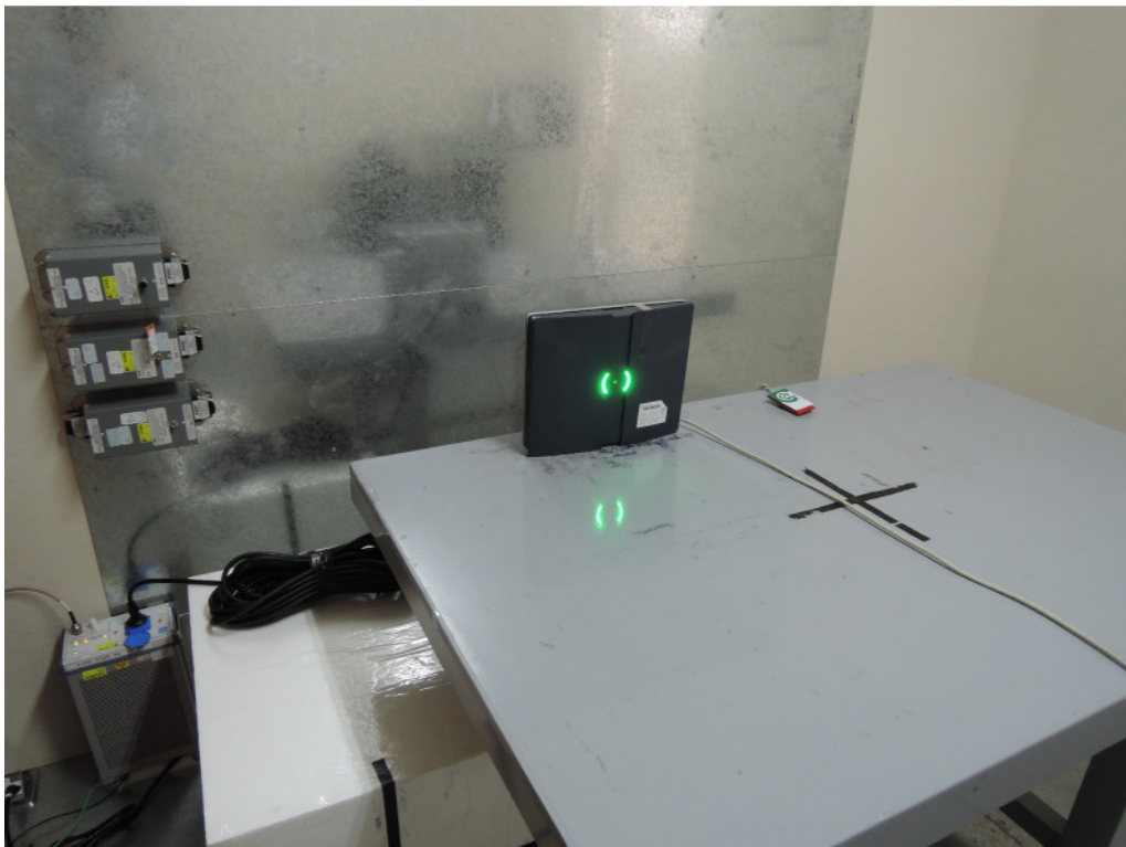
Photograph 5: Set-up for for Mains Conducted testing Front
