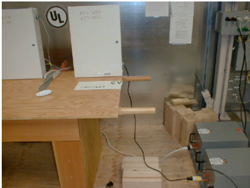
Figure 6.1 - Conducted Voltage Emissions Measurement Configuration (AL-1191)
