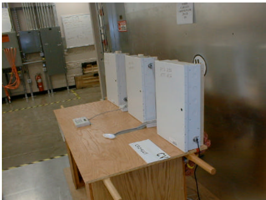
Figure 6.2 - Conducted Voltage Emissions Measurement Configuration (AL-1191)
