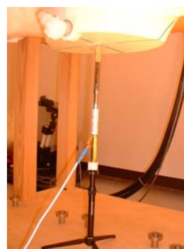
2450MHz System performance check setup
