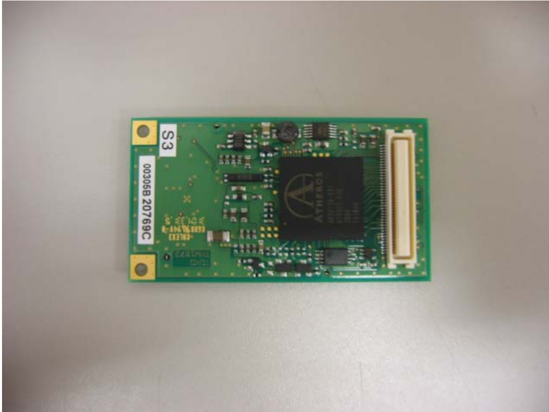
Rear of Wireless LAN module (with shielded)
