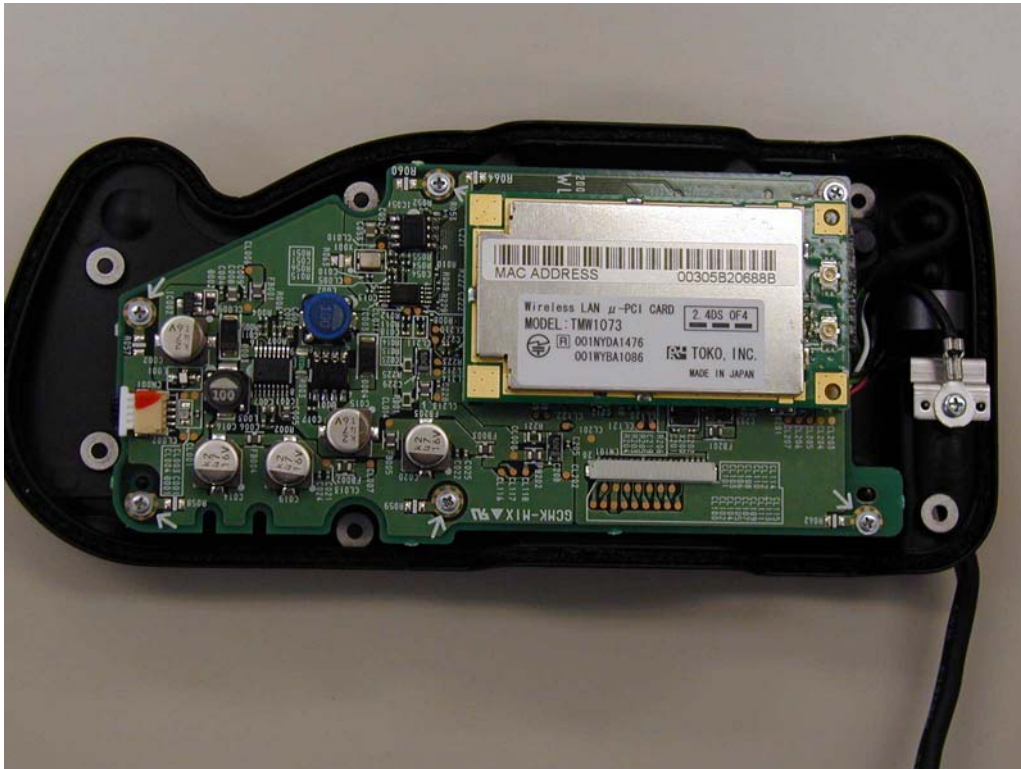
Wireless Transmitter Cover Opened (without cover)
