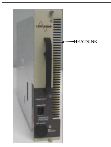
Figure 12: Power amplifier segment heatsink.
