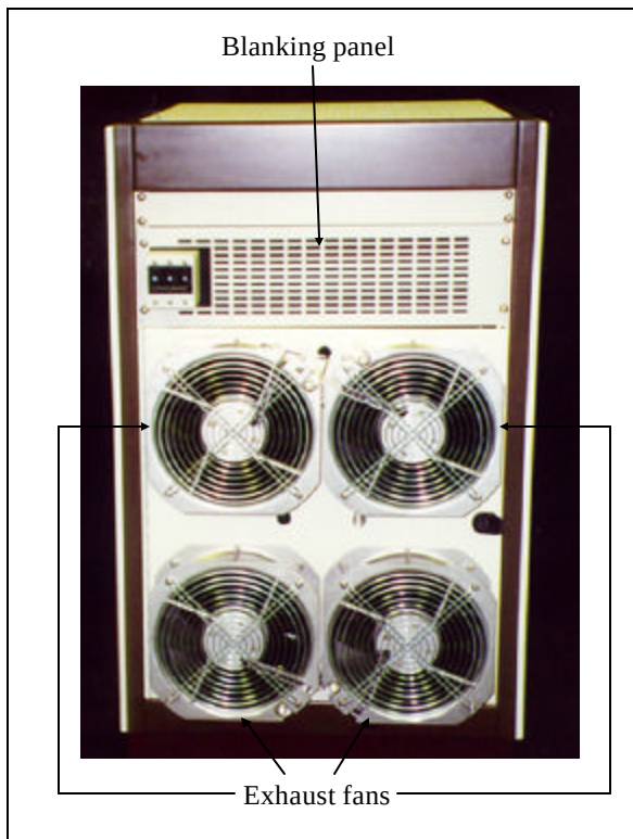
Figure 13: Blanking panel & exhaust fans.
