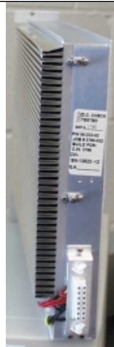
Figure 10: Power amplifier segment rear panel.
